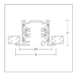
Aluminium extrusion profile painted, tracks can be cut to any required length, may be used within hand's reach, with five mounting holes at 100, 990, 1990, 2990, 3875mm.
