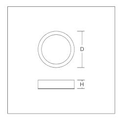
Flexible round surface-mounted multifunction downlight. Luminaire for escape route illumination. Housing: die-cast aluminium, powder-coated. Diffuser made of non-yellowing plastic (PMMA) microprismatic. Suitable for Ceiling mounting, Wall (surface). Self-contained system with automatic self-test and feedback via DALI bus, only to RZB DALI monitoring system.
