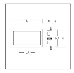
Luminaire for escape route identification. Housing: anodised aluminium, silver. Display panel: patented MicroLens technology and legend on one side. Electronic ballast included. Self-contained system with automatic self-test. Please indicate legend number when placing your order!
