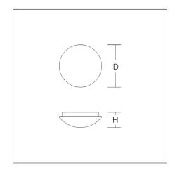
Decorative round surface-mounted luminaire for indoor and outdoor use. Base: plastic. Diffuser made of non-yellowing plastic (PMMA), opal. Diffuser fastening: spring system. Suitable for Ceiling mounting, Wall (surface). Slave luminaire. Can only be operated in combination with corresponding master luminaire. IP 43 ceiling mounting, IP 44 wall mounting.
