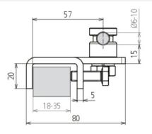
Heavy design; for connection to steel structures.
