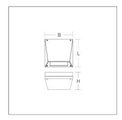
Wall luminaire for escape route illumination. Housing: die-cast aluminium, powder-coated. With plastic lenses for escape route illumination. Driver integrated. Suitable for connection to central battery systems.
