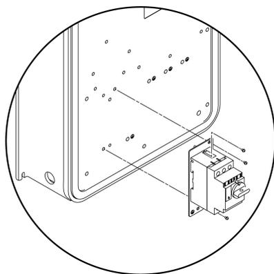
These drives can be equipped with an optional GV2 circuit-breaker, using the optional base plate VW3A9922 and rotary handle GVAPB65S, supplied with detailed mounting instruction sheet PHA63344.
