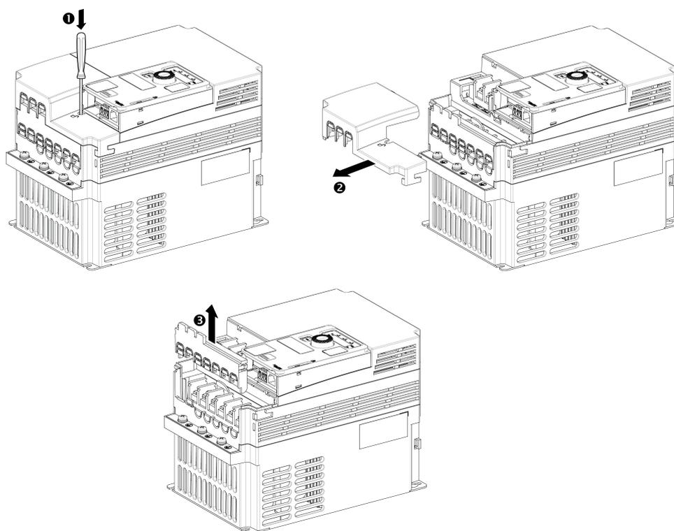
Apply the following instructions to access the power terminals on **frame sizes 4C** drives:
