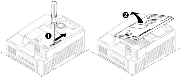
Control block of ATV320●●●●●C and ATV320●●●●●W(S) can be removed to facilitate the wiring.
