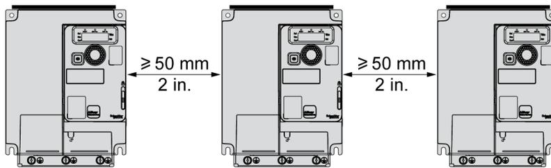
Free space  $\geq 50$  mm (2 in.) on each side, with vent cover fitted.
