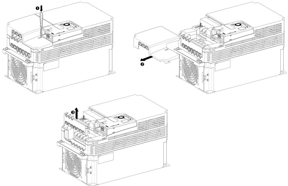
Apply the following instructions to access the power terminals on **frame sizes 5C** drives:
