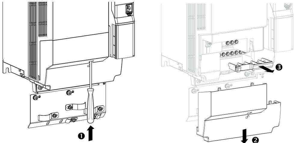
Apply the following instructions to access the power terminals on **frame sizes 4B and 5B** drives:
