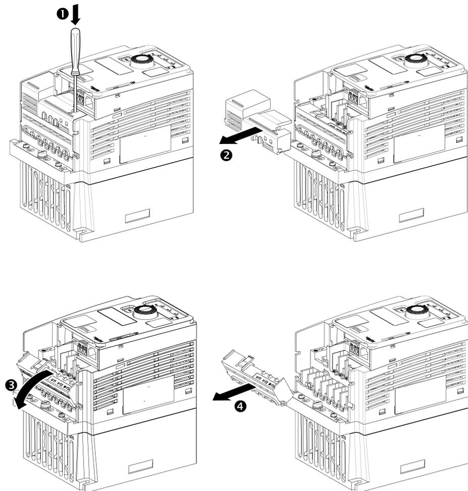
Apply the following instructions to access the power terminals on **frame sizes 2C** drives:
