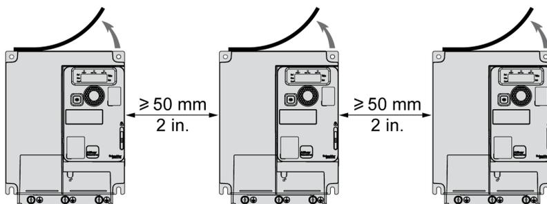
Free space  $\geq 50$  mm (2 in.) on each side. Vent cover should be removed for operation at surrounding air temperature above 50 °C (122 °F). The degree of protection becomes IP20.
