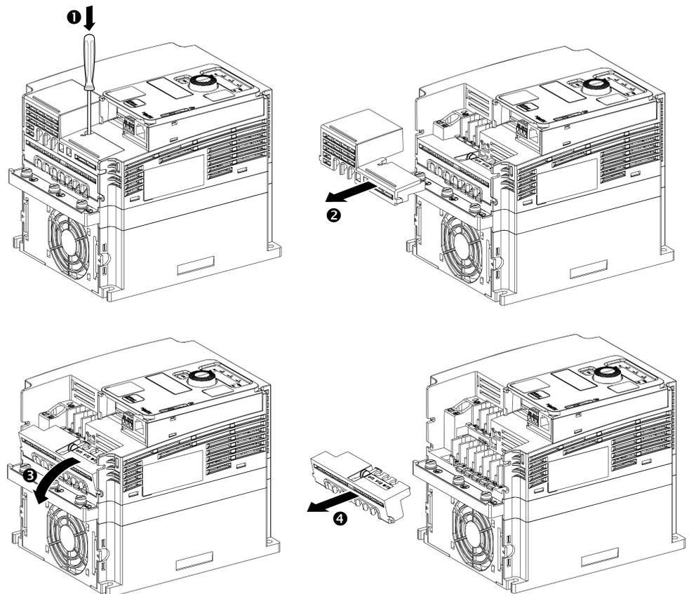
Apply the following instructions to access the power terminals on **frame sizes 3C** drives:
