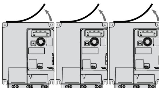
Drives mounted side-by-side, vent cover should be removed. The degree of protection becomes IP20.
