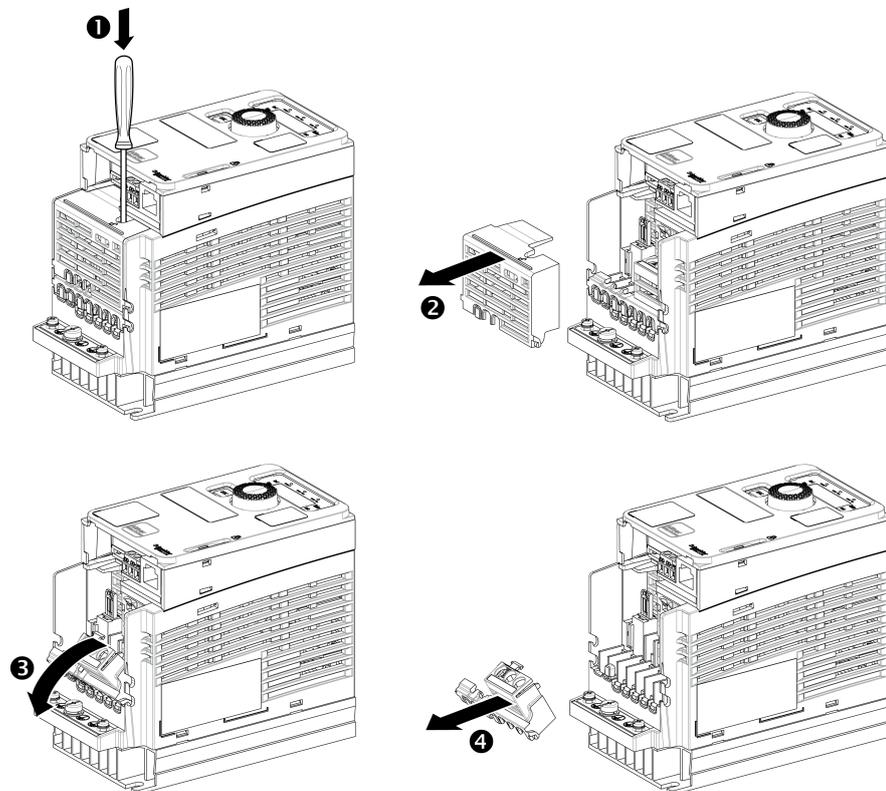
Apply the following instructions to access the power terminals on **frame sizes 1C** drives:
