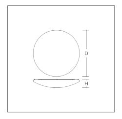
Decorative round surface-mounted luminaire. For escape route illumination. Base: metal, powder-coated. Diffuser made of non-yellowing plastic (PMMA), opal. Diffuser fastening: patented push system. Suitable for Ceiling mounting, Wall (surface). Self-contained system with automatic self-test and feedback via DALI bus, only to RZB DALI monitoring system.
