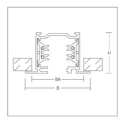
Aluminium extrusion profile, lacquered, can be cut to any length. May be used within hand's reach. With three fixing holes at 100, 990, 1880mm.
