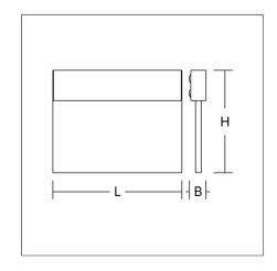
Luminaire for escape route identification. Housing: extruded aluminium profile, anodised or powder-coated. Display panel: highly transparent plastic, with motifs on one side. Electronic ballast included. Self-contained system with automatic self-test and feedback via DALI bus, only to RZB DALI monitoring system. Please indicate legend number when placing your order!
