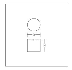
High-quality surface-mounted downlight for indoor and outdoor use. Housing made of corrosion-resistant die-cast aluminium, seawater resistant powder-coated. With membrane valve as a standard to avoid condensed water. Cover clear single-pane toughened glass. Rotation-symmetric reflector made of reflex-boosted MIRO-SILVER®. Easy installation with a separate ceiling frame and plug connection.. 5 pole double terminal for through-wiring.
