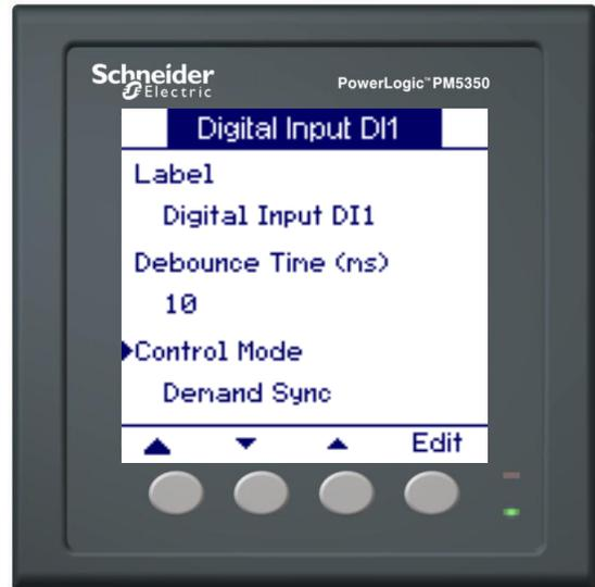
When using a digital input for demand sync, the selected demand method must be “Input Synchronized Block,” or “Input Synchronized Rolling Block,” and the demand interval duration and demand subinterval duration configurations must be the expected durations. The demand sync pulse from the external meter must occur within +/- 5 seconds of the expected duration to be considered a valid sync pulse.
