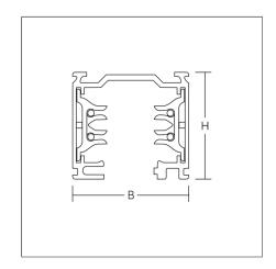
Aluminium extrusion profile painted, tracks can be cut to any required length, may be used within hand's reach, with two mounting holes at 100, 880mm.
