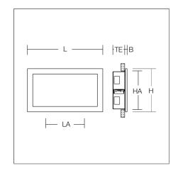
Luminaire for escape route identification. Housing: anodised aluminium, silver. Display panel: patented MicroLens technology and legend on one side. Electronic ballast included. Self-contained system with automatic self-test and feedback via DALI bus, only to RZB DALI monitoring system. Please indicate legend number when placing your order!
