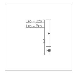
Luminaire tube with anchoring tube. Height 4200 mm. Luminaire tube made of aluminum profile, seawater resistant powder-coated. Continuous buried base with two side cable holes. Including fastening screws for cable fuse box. Pole door with triangle lock. Luminaire tube height 3200 / 3700 mm on request.
