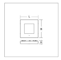
Flat, square surface-mounted luminaire. Base: die-cast aluminium, powder-coated Cover: polycarbonate. With narrow beam plastic lenses for escape route lighting. Suitable for connection to central battery systems. Luminaires with limited surface temperature in accordance with EN 60598-2-24 for use in environments in which a deposit of conductive dust on the luminaire can be expected. Ball impact proof in accordance with DIN 18032-3. Qualified for use in the food and drink industry.
