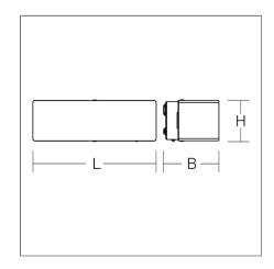
Luminaires for escape route identification Base: metal, powder-coated. Diffuser: plastic (polycarbonate), opal. 4 plastic foils with escape route motifs included (ISO 7010). Electronic ballast included. Self-contained system with automatic self-test and feedback to the RZB monitoring system MULTIDIGIT.
