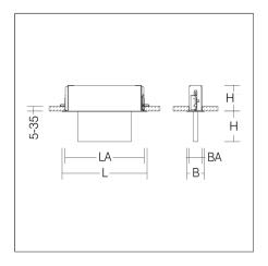
Luminaire for escape route identification. Installation housing sheet steel. Ceiling plate stainless steel high polish or powder-coated. Display panel: highly transparent panel, plastic, with legend on one side/both sides. Driver integrated. Suitable for connection to central battery systems. Please indicate legend number when placing your order!
