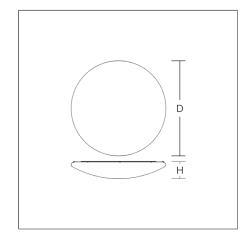
Decorative round surface-mounted luminaire. For escape route illumination. Base: metal, powder-coated. Diffuser made of plastic (polycarbonate), opal, shockproof. Diffuser fastening: patented push system. Suitable for Ceiling mounting, Wall (surface). Electronic ballast included. Self-contained system with automatic self-test.
