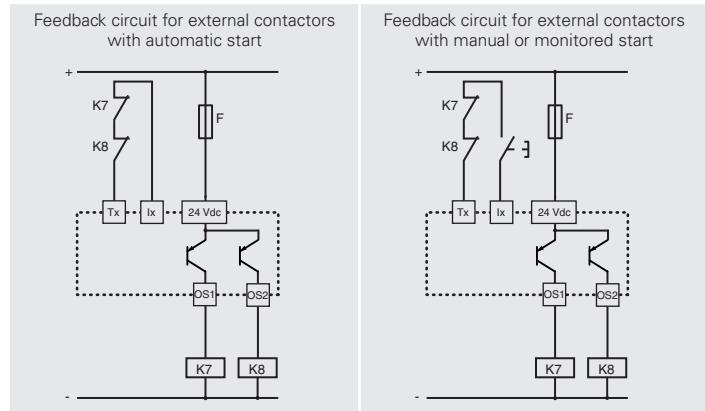
In order to function correctly, any modules or PLCs connected to the OSx safety electronic outputs must be able to withstand cyclical deactivation tests performed on the same.
