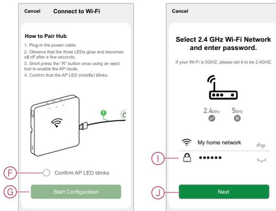
8. (See K) Once the Wi-Fi connection is successful with the gateway, a hotspot network will be created with the Wi-Fi name **WiserGW\_XXXXXX** (I). Tap **Go to Connect** (See L).
