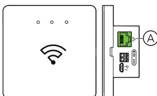
2. Connect an Ethernet cable between the gateway and the router to suit the installation method used for the gateway:
