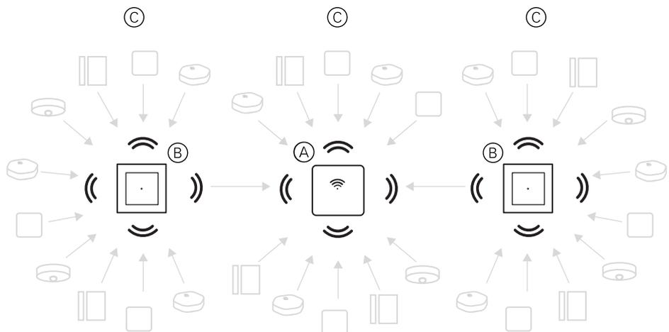
**TIP:** Install and commission all mains-powered devices before commissioning battery-powered devices. This provides maximum hosting capacity prior to adding the battery-powered devices.
