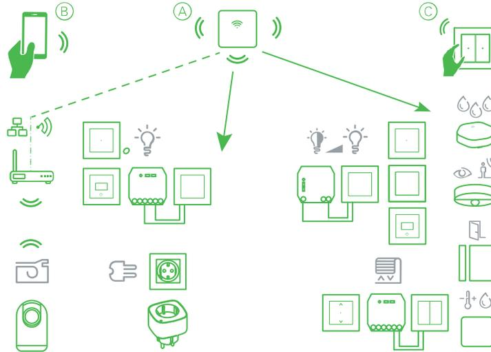
The Wiser gateway (see A) is the center of the system, processing control requests and status reports for connected Wiser devices.
