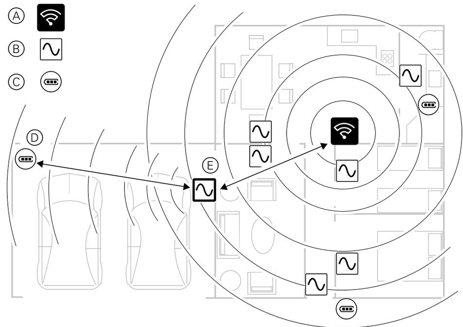
**TIP:** The battery-powered motion sensor in the garage (D) is a long way from the gateway. However, the sensor can connect to the gateway via the mains-powered device being used as the garage light switch (E). This is because mains-powered devices also act as system network extenders. Consider this when deciding where to locate the gateway.
