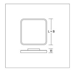
Decorative square LED surface-mounted luminaire. Flat, seamless frame: aluminium extrusion profile, powder coated. Cover made of sheet steel, powder-coated. Diffuser made of non-yellowing plastic (PMMA), opal. LED backlight technology for homogeneous illumination of the entire light-emitting surface. Suitable for Ceiling mounting, Wall (surface). Very easy installation thanks to plug & play connection. Driver integrated. Dimmable DALI. Suitable for through-wiring.
