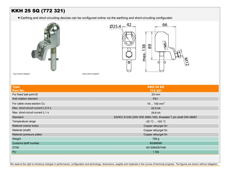
The clamps must have the same maximum short-circuit current as the earthing and short-circuiting cables!
