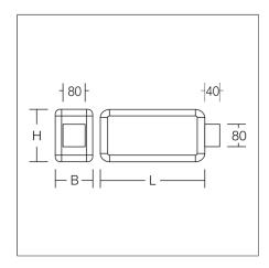
Rectangular wall extension luminaire in classic design. For escape route identification. Housing: aluminium, with plastic corner connectors. Display panels: plastic, opal, with motifs on one side/on both sides. Wall extension Electronic ballast included. Self-contained system with automatic self-test. Please indicate legend number when placing your order!
