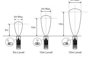
Point the remote facing forward towards the motion sensor of the Highbay MD, all the luminaires with sensor within range will respond to the signal.
