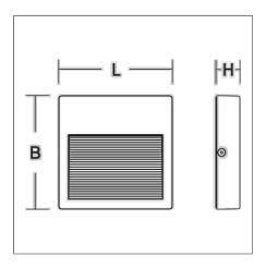
Flat surface-mounted LED fitting for illumination of wall related areas such as stairs, ramps or corridors. Housing made of corrosion-resistant die-cast aluminium, powder-coated. Stainless steel screws. Diffuser with clear toughened glass. Asymmetrical downward light distribution for wide dispersion and uniform illumination. With compensation for drill hole deviations. Driver integrated. With connecting terminal up to  $1 \times 3 \times 1.5 \text{ mm}^2$ , for max. 13 mm diameter mains cable.
