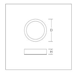
Flexible round surface-mounted multifunction downlight. Luminaire for escape route illumination. Housing: die-cast aluminium, powder-coated. Light guide and diffuser made of non-yellowing PMMA, opal matt. Suitable for Ceiling mounting, Wall (surface). Driver integrated. Suitable for connection to central battery systems.
