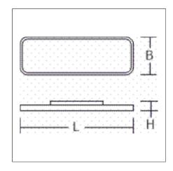
Decorative rectangular LED surface-mounted luminaire. Flat, seamless frame: aluminium extrusion profile, powder coated. Cover made of sheet steel, powder-coated. Diffuser made of non-yellowing plastic (PMMA), opal. LED backlight technology for homogeneous illumination of the entire light-emitting surface. Suitable for Ceiling mounting, Wall (surface). Very easy installation thanks to plug & play connection. Driver integrated. Dimmable DALI. Suitable for through-wiring.
