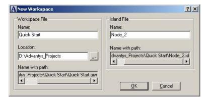
In our example, we have chosen the path D:\Advantys\_Projects\Quick Start. The name of the project file is Quick Start.aiw and the name of the Advantys STB is Node\_2 (referring to its CANopen node address). All the Advantys STB on the same bus must be declared in the same workspace. The Default workspace path is C:\program Files\Schneider Electric\Advantys\Project\
