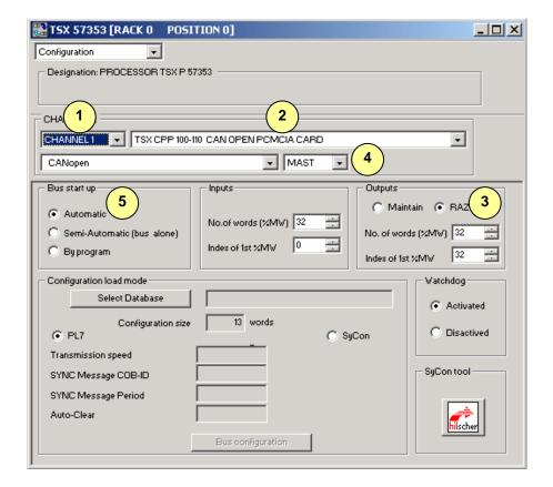
Start PL7, configure the hardware and double click on the PCMCIA slot of the CPU
