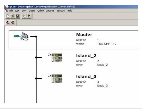
SyCon tool - Step 5 Set the Baud rate to 250 kBit Simply Click on the TSX CPP 110 and then select **Settings->Bus Prameter** in the menu. Change the Baud rate to 250 kBit/s, the value previously set on the Advantys STB hardware.
