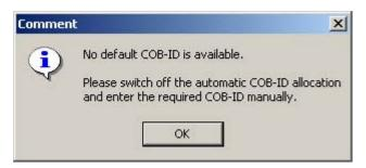
Disable the automatic COB-ID allocation (node configuration screen). Now you can manually overwrite the COB-ID for PDO5, PDO6, ...
