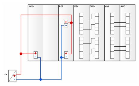
Note that we recommend having a separate power supply for the outputs. For testing purposes, however, you can have one common power supply for inputs, outputs and logic supply (as shown in the figure above).
