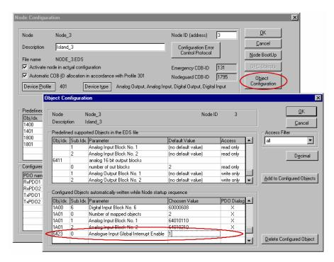
Close the window and save the project. You have now finished the CANopen configuration with SyCon and created the necessary data required by PL7 to configure the TSX CPP110 module.
