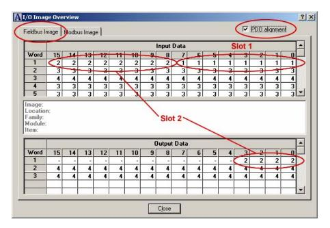
Do the same for Node #2. Make a hardcopy of both screens as it helps in understanding the IO mapping.
