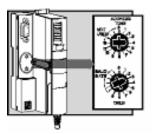
Both the baud rate and the node address are set using the two rotary switches in the middle of the NCO module.
