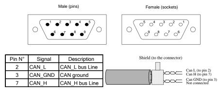
Pins 2, 3, and 7 must be connected.
