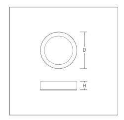
Super-flat surface mounted downlight for high requirements. Cylinder housing sheet steel, powder-coated. Bezel ring: die-cast aluminium, powder-coated. Diffuser made from resistant polycarbonate (PC) with smooth surface on room side for low sensitivity to dirt and for the prevention of the accumulation of germs and bacteria. Satinised microprismatic diffuser prevents direct glare. Suitable for Ceiling mounting, Wall (surface). Driver integrated. Cyanosis Observation Index (COI) <3.3.
