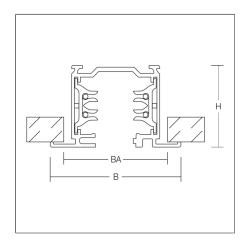
Aluminium extrusion profile painted, tracks can be cut to any required length, may be used within hand's reach, with three mounting holes at 100, 990, 1880mm.
