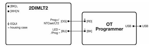
The new programmed parameters would get valid with the next power on cycle. Further details are available in the application guide for the 2DIMLT2 family.
