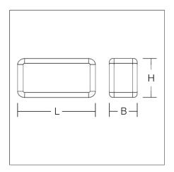
Luminaire for escape route identification. Housing: aluminium, with plastic corner connectors. Display panel: plastic, opal, with legend on one side. Electronic ballast included. Self-contained system with automatic self-test. Please indicate legend number when placing your order!
