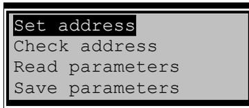
Choose the "Set address" start menu – scroll with "UP" and "Down" buttons if necessary.
