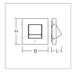
Wall luminaire for escape route illumination. Base: die-cast aluminium, powder-coated Cover: polycarbonate. With plastic lenses for area lighting. Vertical swivel. Electronic ballast included. Self-contained system with automatic self-test and feedback via DALI bus, only to RZB DALI monitoring system. Luminaires with limited surface temperature in accordance with EN 60598-2-24 for use in environments in which a deposit of conductive dust on the luminaire can be expected.
