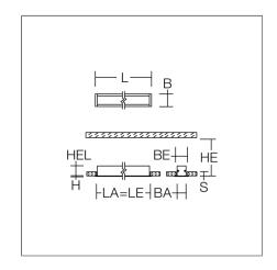
Recessed ceiling and wall luminaire with slim design. Housing: extruded aluminium profile, powder-coated. End cap aluminium powder-coated. High polish aluminium micro grid. Perfect for office areas (UGR ≤ 19) and environments with computer screens in accordance with EN 12464-1. Suitable for Recessed ceiling mounting, wall (recessed). External driver with connecting cable.
