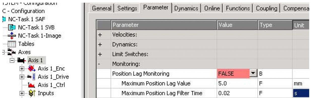
If you use the operating mode Cyclic Synchronous Position, set "Position Lag Monitoring" to "FALSE".
