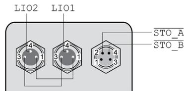
Pin 1 is internally connected to CN4.1 (+24VDC\_OUT).
