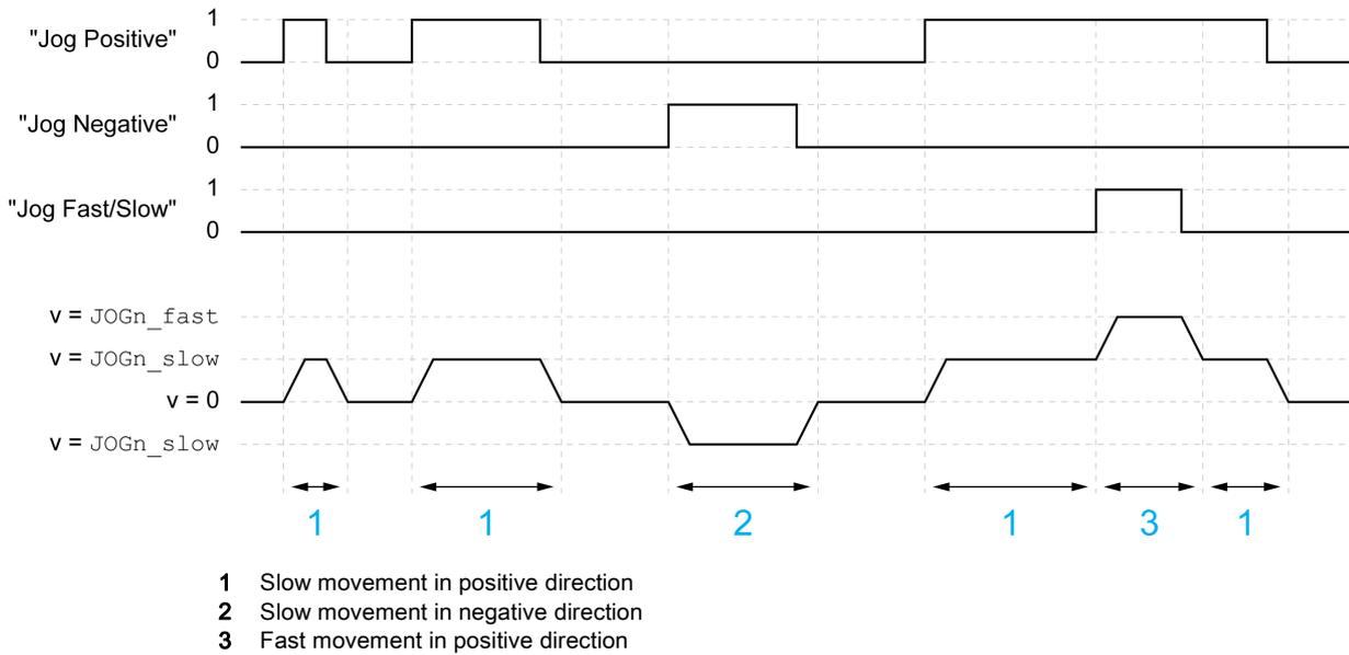
The illustration below provides an example of continuous movement via the fieldbus:
