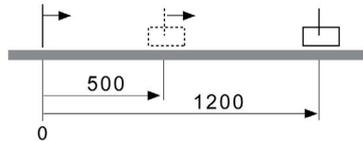
A zero point must be defined with the operating mode Homing prior to the first absolute movement.
