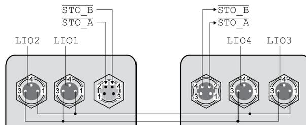
Pin 1 is internally connected to CN4.1 (+24VDC\_OUT).
