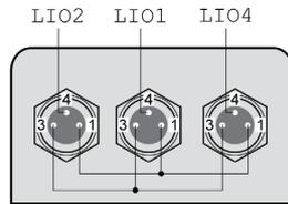
Pin 1 is internally connected to CN4.1 (+24VDC\_OUT).
