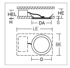
Super-flat recessed downlight for high requirements. Housing: die-cast aluminium. Diffuser made from resistant polycarbonate (PC) with smooth surface on room side for low sensitivity to dirt and for the prevention of the accumulation of germs and bacteria. Satinised microprismatic diffuser prevents direct glare. Ceiling installation with spring system. Mounting depth depends on ceiling strength. Suitable for throughwiring. Including separate LED converter with connecting cable 250 mm.
