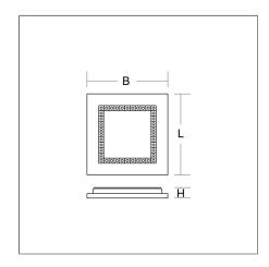
Glare-free LED ceiling luminaire with optical lens system. Base: metal, powder-coated, with bayonet fixing. Housing: plastic (polycarbonate). Housing and diffuser are screwed together. Diffuser with optic lenses. Big terminal block; ideal for through-wiring. Sealing strip on the back of the luminaire connects seamlessly with the ceiling. Easy installation with Plug & Play plug connection. Thanks to UGR < 22 ideal for corridors, stairways, shops, schools, meeting rooms, rest areas.
