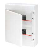
The IP40 protected decorative enclosures are available in sizes from 8 to 72M. They provide superior aesthetic integration and are equipped with screw wiring multipolar terminal blocks, 80 A IP 20. They are available with smoked transparent doors or with blank doors that can be equipped with safety lock, characterized by the "PUSH" opening and closing. The terminal blocks allow to create simple and neat wiring reducing the set-up time of the enclosure.
