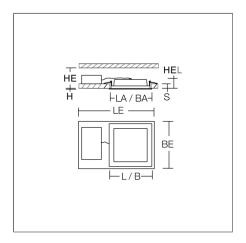
Flexible square recessed multifunction downlight. Luminaire for escape route illumination. Housing: sheet steel, powder-coated. Luminaire frame: aluminium, powder-coated. Diffuser made of non-yellowing plastic (PMMA), opal. LED backlight technology for homogeneous illumination of the entire light-emitting surface. Ceiling installation with spring system. Including separate LED converter with connecting cable 250 mm.
