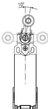
For switches with swivelling lever, the lever can be adjusted in 10° steps over the entire 360° range. The positive movement transmission is always guaranteed thanks to the particular geometrical coupling between the lever and the revolving shaft as prescribed for safety applications by the German standard BG-GS-ET-15.
