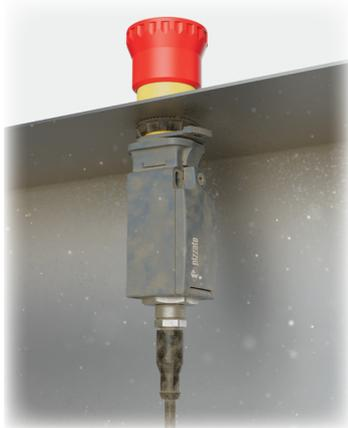
Protected contact block for control devices fitted in switching cabinets with the presence of dust also inside the cabinet. The block ensures an IP67, IP69K protection degree for internal electric contacts.
