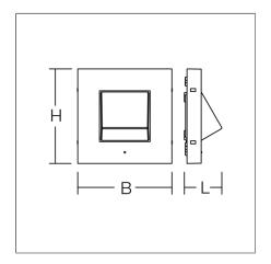
Wall luminaire for escape route illumination. Base: die-cast aluminium, powder-coated Cover: polycarbonate. With plastic lenses for escape route illumination. Vertical swivel. Driver integrated. Suitable for connection to central battery systems. Luminaires with limited surface temperature in accordance with EN 60598-2-24 for use in environments in which a deposit of conductive dust on the luminaire can be expected.
