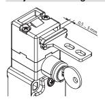
The actuation head of this switch features a wide range of travel. In this way the guard can oscillate along the direction of insertion (4.5 mm) without causing unwanted machine shutdowns. This wide range of travel is available in all actuators in order to ensure maximum device reliability.
