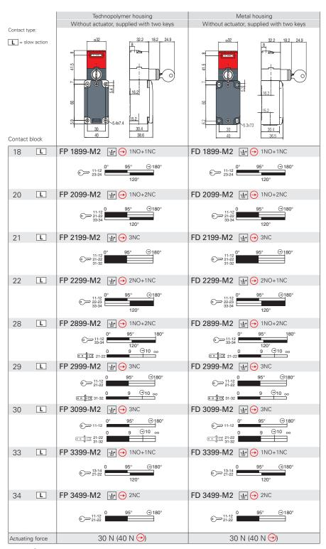
Legend: With positive opening according to EN 60947-5-1, 12 interlock with lock monitoring acc. to EN ISO 14119
