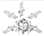
The head can be guickly turned to each of the four sides of the switch by unfastening the two fastening screws.
