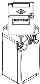
To make head adjustment safer and smoother, these switches are equipped with a special head to body coupling system. This system makes it impossible to remove the head from the device even during adjustment, thus rendering the use of one-way screws unnecessary for locking the head in position once adjustment is complete. This solution is available for the FR, FX and FK series.
