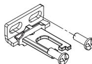
As required by EN ISO 14119, the actuator must be fixed immovably to the guard frame. Pan head safety screws with one-way fitting are available for this purpose. With this screw type, the actuators cannot be removed or tampered with using common tools. See accessories on page 419.
