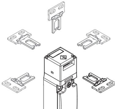
For all switches, the head can be adjusted in 90° steps after removing the two fastening screws. In this way it is possible to actuate the switch from 5 different directions.
