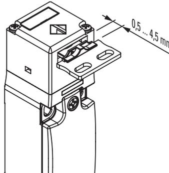
The actuation head of this switch features a wide range of travel. In this way the guard can oscillate along the direction of insertion (4 mm) without causing unwanted machine shutdowns. This wide range of travel is available in all actuators in order to ensure maximum device reliability.
