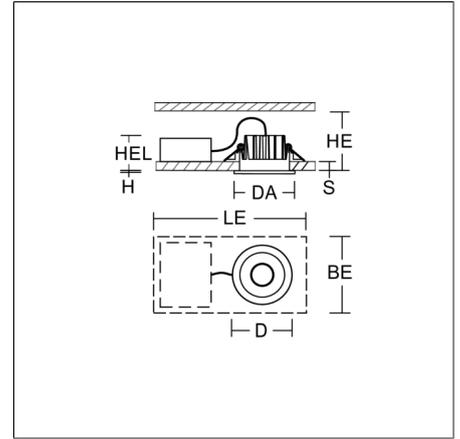
Round emergency luminaire for escape route lighting. With asymmetrical beam plastic lenses for illuminating rescue facilities. Suitable for connection to central battery systems. With enclosed separate ceiling mounting ring also suitable for ceiling cut-outs of Ø 68 mm.
