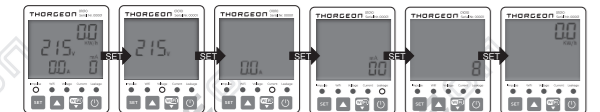
○ Function display ○ Undervoltage/Overvoltage Setting ○ Overcurrent Setting ○ Leakage Setting (This feature can be turned off) ○ Self-Reset Time Setting ○ Power Meter
