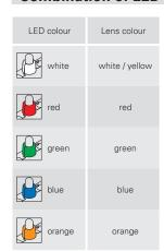
**Note:**Combinations of LED colour with lens colour different from the recommended ones can give a different colour compared to the expected one.
