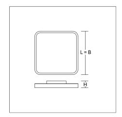
Decorative square LED surface-mounted luminaire. Flat, seamless frame: aluminium extrusion profile, powder coated. Cover made of sheet steel, powder-coated. Diffuser made of non-yellowing plastic (PMMA), opal. LED backlight technology for homogeneous illumination of the entire light-emitting surface. Suitable for Ceiling mounting, Wall (surface). Very easy installation thanks to plug & play connection. Driver integrated. Dimmable DALI. Suitable for through-wiring.
